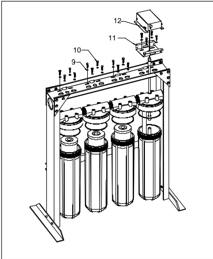
**Figure 5:** Module Attachment Points
